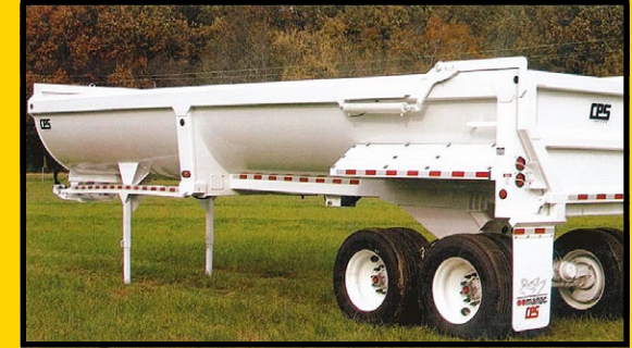
2012 CPS Half Round End Dump 32' x 102", Single Point Suspension, Tandem Fixed Axle, All Steel Wheels, New 2012 CPS Half Round End Dump On Order Will Arrive End Of June.
