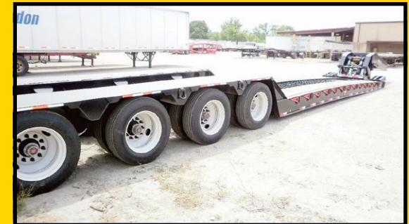
2012 PITTS 55 ton detachable neck lowboy 58' x 102", Air Ride Suspension, Quad Fixed Axle, All Steel Wheels, Apitong Floor, 55 Ton Detachable Neck Lowboy 4 axles Call For Price We Want Your Trade ..... Any Make or Model
