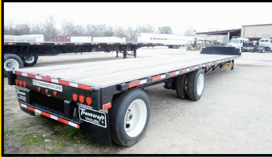
2012 TRANSCRAFT 48' x 102", Air Ride Suspension, Tandem Spread Axle, 255/70R 22.5 Tires, All Steel Wheels, Apitong Floor..... CALL FOR PRICE
